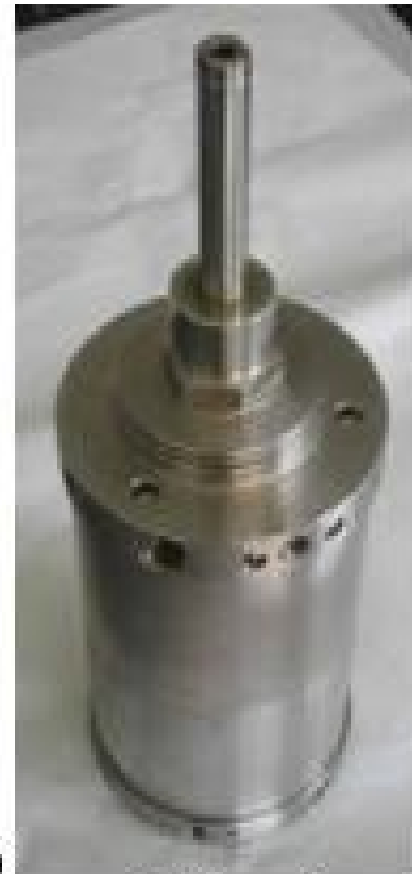
Fig. 1. (a) THM reactor without piston and removable cover, (b) Overview of the THM machine
