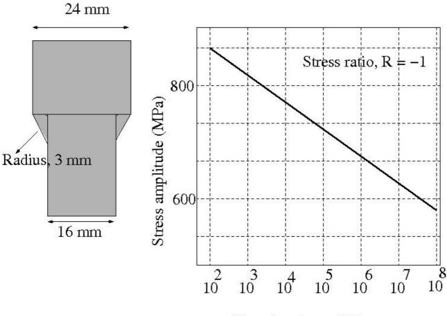
No. of cycles to failure
